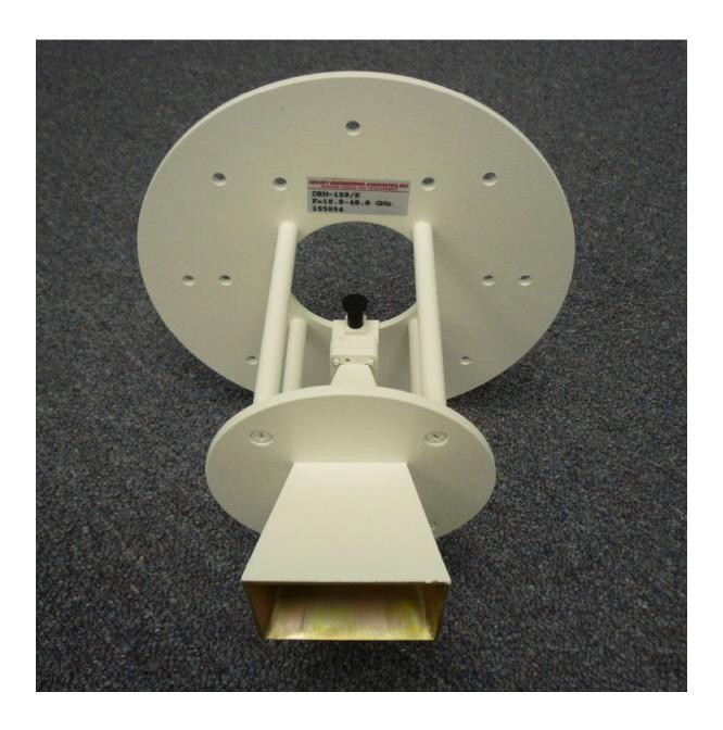
The DRG-1840-A is a linearly-polarized wide-band dual-ridged horn antenna. It is designed to transmit or receive in the frequency band from 18 GHz to 40 GHz. The antenna has high gain, uniform E-Plane and H-Plane radiation patterns, and low VSWR.
