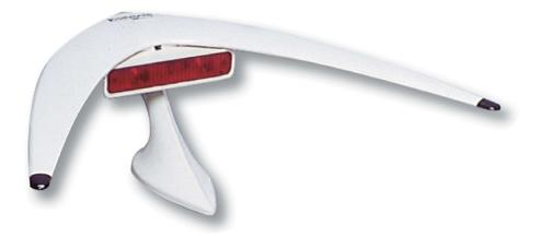
The most classic style of boomerang we offer witha third brake light that provides enhanced visual safety. Simply add a signal amplifier, and you are ready to receive the best signal possible. Ideal for use on your limousine, motor coach, or boat.
