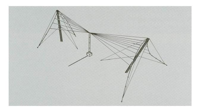
The 1765 antennas require no tuning or resistive loading circuitry. This permits complete compatibility with multichannel fixed-tuned radios as well as frequency agile, synthesized HF radio equipment. Elimination of the antenna coupler maximizes the power output of the antenna/transmitter, resulting also in a significant improvement in communication reliability through the reduction of maintenance and/or repair.
