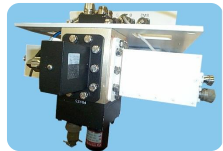
1:1 REDUNDANT LNA SYSTEM
