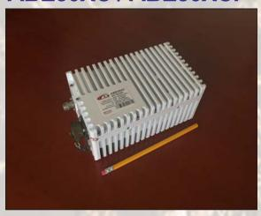
This smallest and lightest fanless 30W(min) L-To C-Band Block Up Converter is based on GaN technology. It could be mounted directly on a feed horn. The unit covers all three C-Band sub-bands: Standard (5.85-6.425 GHz), Palapa (6.365-6.725 GHz) and Insat (6.725-7.05 GHz).
