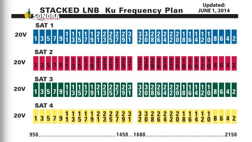
Stacked LNBs' are used by multiple DBS operators. The figure above is the transponder layout for high side inverted stacking of the even polarity. Note that the highest frequncy even transponder is #2.
