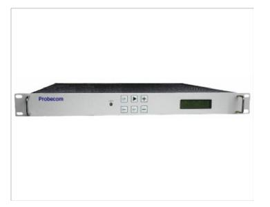
A tracking receiver for antenna step tracking and automatic uplink power control!The Models 3430-L, LD, LF, andLW are fully frequency agile satellite receivers designed to provide a linear DC reference voltage proportional to the received signal level of a satellite beacon or narrow-bandSCPC carrier. Frequency selection on 10 kHz steps may be accomplished from the front panel or remote control. Pre-detection noise bandwidth of 50 kHz facilitates accurate tracking at very low C/N levels.
