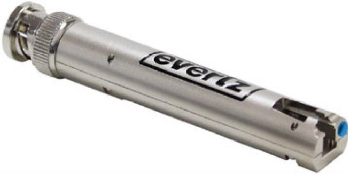
The 2307LR is a fiber optic receiver in a revolutionary form factor. With the same diameter as a BNC connector, and overall length of 3.3" (85mm), the 2307LR is the smallest RF optical receiver in the industry. It accepts an optical LC connector input on one end, and provides an electrical output on the other.
