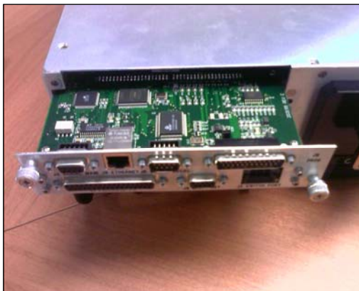
Removable rear panel monitor and control card
