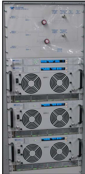
500W X-Band, 1:2 Redundant System in the 4RU chassis, with N+1 redundant power supplies
