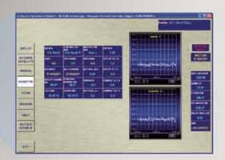
Antenna control system offers optional GUI, built-in spectrum analyzer, monitor and control (including modem) and tracking
