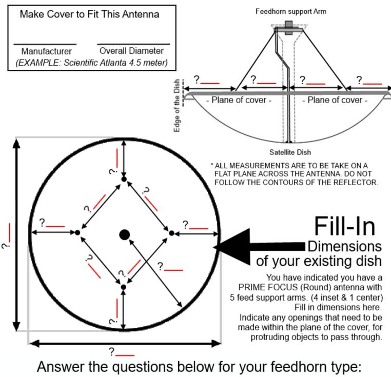
PRIME FOCUS FEEDS (located in front/center of dish)
