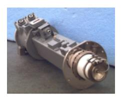
The VTX-5786J family of pulsed-coupled cavity TWTs covers 9.45 GHz to 9.95GHz the 5786J has 12 kW peak output power, 10.0 % duty cycle. This device has a non-intercepting grid pulsed and dual stage depressed collector to achieve 40 dB gain. Custom configurations are also available. These variations in the performance and configuration include: cooling method (affects average power level), mechanical configuration, electrical and RF connections, & single stage depressed collector
