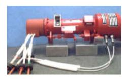
The VTX-5783G pulsed-coupled cavity TWT covers 9.35GHz to 10.1GHz with 50 kW peak output power, 1.0 % duty cycle. This device has a non-intercepting grid pulsed and dual stage depressed collector to achieve 49 dB gain. Custom configurations are also available. These variations in the performance and configuration include: cooling method (affects average power level), mechanical configuration, electrical and RF connections, & single stage depressed collector
