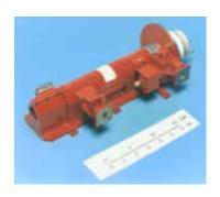
The VTU-5690A pulsed- coupled cavity TWT covers 16.0 GHz to 17.0 GHz with 40 kW peak output power, 0.3 % duty cycle. This device has cathode pulsed and grounded collector to achieve 48 dB gain. Custom configurations are also available. These variations in the performance and configuration include: grid modulation, cooling method (affects average power level), mechanical configuration, electrical and RF connections.
