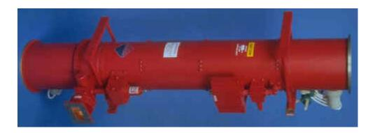
The VTS-5755 pulsed-coupled cavity TWT covers 2.7 GHz to 3.1 GHz with 60 kW peak output power, up to 2.4% duty cycle. This device has a non-intercepting grid pulsed and single stage depressed collector to achieve 50 dB gain. This device is capable of parallel operation from a common HV power supply, phase tracking is better than +/- 20 degrees. The long life CD coated cathode is capable of pulse width to 50 micro seconds in this PPM focused, air cooled TWT
