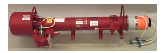
The VTS-5754G pulsed-coupled cavity TWT covers 2.7 GHz to 3.1 GHz with 160 kW peak output power, up to 6% duty cycle. This device has a non-intercepting grid pulsed and single stage depressed collector to achieve 48 dB gain. This device is capable of parallel operation from a common HV power supply, phase tracking is better than +/- 20 degrees. The long life CD coated cathode is capable of pulse width to 200 micro seconds.
