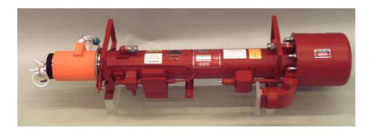
The VTS-5754F pulsed-coupled cavity TWT covers 3.1 GHz to 3.6 GHz with 160 kW peak output power, up to 8% duty cycle. This device has a non-intercepting grid pulsed and single stage depressed collector to achieve 48 dB gain. This device is capable of parallel operation from a common HV power supply, phase tracking is better than +/- 20 degrees. The long life CD coated cathode is capable of pulse width to 200 micro seconds in this PPM focused TWT
