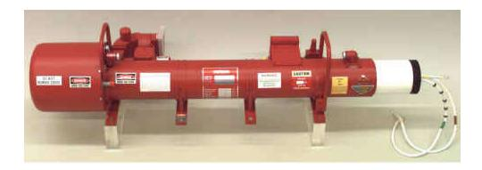
The VTS-5754A pulsed-coupled cavity TWT covers 2.9 GHz to 3.2 GHz with 160 kW peak output power, up to 8% duty cycle. This device has a non-intercepting grid pulsed and single stage depressed collector to achieve 48 dB gain. This device is capable of parallel operation from a common HV power supply, phase tracking is better than +/- 20 degrees. The long life CD coated cathode is capable of pulse width to 200 micro seconds in this PPM focused
