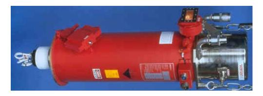
The VTS-5753 pulsed-coupled cavity TWT covers 3.1 GHz to 3.5 GHz with 170 kW peak output power, up to 16% duty cycle. This solenoid focused device has a non-intercepting grid pulsed and single stage depressed collector to achieve 46 dB gain. This device is capable of parallel operation from a common HV power supply, phase tracking is better than +/- 20 degrees. The long life CD coated cathode is capable of pulse width to 1 millisecond.
