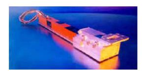
400 Watt, 5.725 - 7.10 GHz, CW traveling wave tube, periodic-permanent-magnet focused, coaxial input, waveguide output, conduction cooled. Custom configurations are also available. These variations in the performance and configuration include: mechanical configuration, electrical and RF connections, and dual-stage depressed collector.
