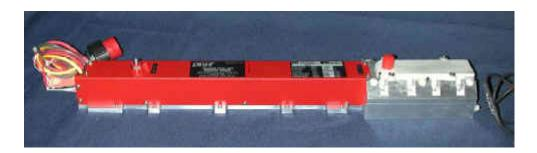
VTC-6260E4 is a 125 W, CW Traveling-Wave Amplifier, 5.850 GHz to 6.425 GHz, Periodic-Permanent-Magnet Focused, Coaxial Input, Coaxial Output, and Conduction Cooled. Custom configurations are also available. These variations in the performance and configuration include: cooling method (affects average power level), mechanical configuration, electrical and RF connections, & single stage depressed collector.
