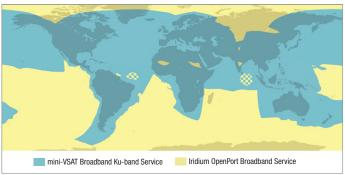
\* The TracPhone V3P is a 2-axis, stabilized antenna that does not provide coverage in areas where the satellite is directly overhead as shown in the hatched areas above. The map depicts KVH's expectations for coverage; actual coverage and availability may vary. Data rates may also vary in different regions. Go to www.kvh.com/minivsatmap to view our coverage map and for complete details. KVH provides no guarantees of satellite coverage or availability.
