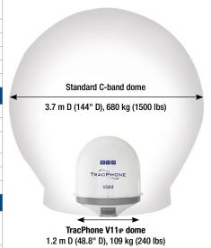
85% smaller in volume and lighter than standard C-band antennas, TracPhone V11₽ is faster, easier, and less expensive to install.
