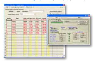
The NetMAC® can monitor any number of carriers for proper C/N ratios, power levels, noise floors, and EIRP.
