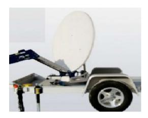
transportable VSAT satellite Internet communication system that provides full functionality for voice and Internet data communications in remote locations. Simply connect the NIMO trailer to your truck and transport it to your field operations site. The auto-pointing system is easy to operate, enabling quick set-up time for voice and data requirements. NIMO is available for purchase or on a monthly rental basis for short-term requirements.
