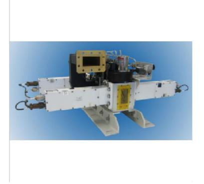
The General Dynamics LRC-1000 Series Redundant LNA systems minimize system downtime due to LNA failure by providing a spare LNA and an automatic means of switching to the spare upon failure of a primary LNA. A 1:1 system provides one spare LNA for one primary LNA. A 1:2 system provides a spare LNA for either of two primary LNAs. The systems consist of an outdoor plate assembly which mounts at the antenna hub, an indoor control panel and interconnecting control cable.
