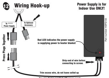
Route the supplied lead wire from the blanket to the power supply location. **TRIM** any excess wire, do not leave excess wire coiled up. Strip both ends and connect to the power supply utilizing the two screw posts. It does not matter which wire you connect to which post. Connect the AC power cord and plug into 120VAC outlet.
