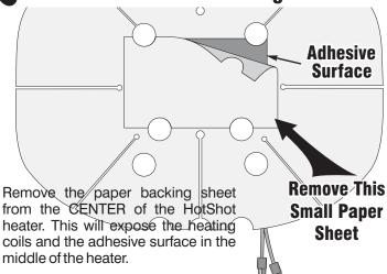
Do Not remove any other protective sheets until you have aligned and attached the heater to your dish.
