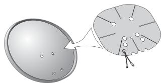
Place the HotShot on the attachment area surface of your dish and lightly press the exposed **center** section adhesive down onto the reflector. Go to step #9 for the completion of the attachment procedure.
