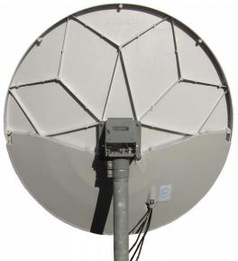
The **Skyware Global Factory-installed Anti-icing System** is designed to keep the reflector and feed horn free from ice and snow during most inclement weather conditions. An automated sensor will energize the reflector and feed horn heaters, when temperatures fall below 3°C (38°F) and when moisture is present. This sensor prevents the system being activated unnecessarily to conserve energy.
