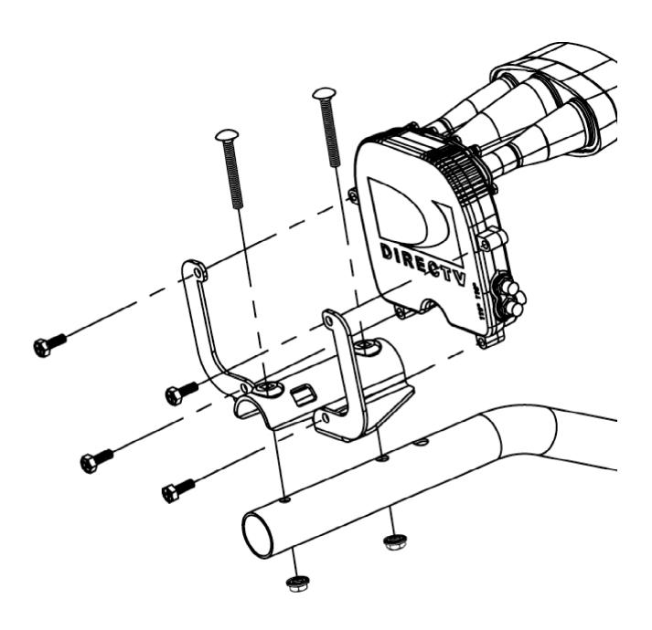
1) Attach LNB mounting bracket to the feed tube as shown, using 2pc 1/4 x 2" carriage
