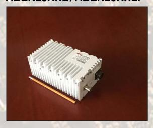
This smallest and lightest fanless 20W L-To Ku-Band Block Up Converter is designed to be mounted on a feed horn. The unit is ideal for portable and mobile applications. Double – L.O. feature makes unit universal for Ku-Band requirements. It is powered either with 24/48 VDC and consumes less than 97W.
