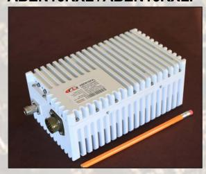
This smallest and lightest fanless 16W L-To Ku-Band Block Up Converter is designed to be mounted on a feed horn. The unit is ideal for portable and mobile applications. Double – L.O. feature makes unit universal for Ku-Band requirements. It is powered either with 24/48 VDC and consumes less than 92W.
