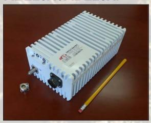
This smallest and lightest fanless 47W L-To X-Band Block Up Converter is based on GaN technology. It could be mounted directly on a feed horn. M&C (FSK) capability enables troubleshooting, monitoring and controlling the BUC. The unit can be powered either with 24VDC or 48VDC. Unit can use either external or internal 10MHz reference.
