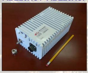
This smallest and lightest fanless 20W(min) L-To C-Band Block Up Converter is based on GaN technology. It could be mounted directly on a feed horn. The unit covers all three C-Band sub-bands: Standard (5.85-6.425 GHz), Palapa (6.365-6.725 GHz) and Insat (6.725-7.05 GHz).
