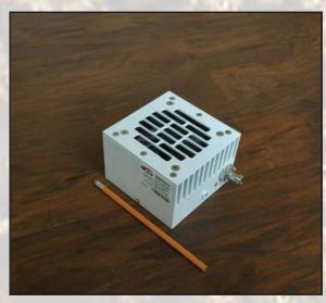
This smallest and lightest 20W L-To Ku-Band Block Up Converter is based on GaN technology. Incomparable low power consumption, double L.O., field-exchangeable connector, internal 10 MHz reference, and it is powered either with 24 or 48 VDC and consumes less than 135W. The unit is ideal for portable and mobile aplications.
