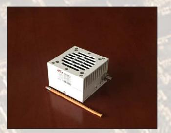
This smallest and lightest 38W L-To Ku-Band Block Up Converter is designed to be mounted on a feed horn. The unit is ideal for portable and mobile applications. Double – L.O. feature makes unit universal for Ku-Band requirements. It is powered either with 24 or 48 VDC and consumes less than 94W.
