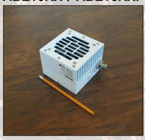
This smallest and lightest 16W L-To Ku-Band Block Up Converter is designed to be mounted on a feed horn. The unit is ideal for portable and mobile applications. Double – L.O. feature makes unit universal for Ku-Band requirements. It is powered either with 24 or 48 VDC and consumes less than 92W.
