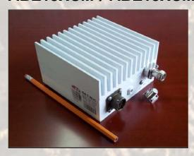
This smallest and lightest 15W L-To C-Band Block Up Converter is based on GaN technology. It is designed to be mounted on the feed horn. High power efficiency resulting in low current (<1 amps @ 48VDC) .The unit covers all three C-Band sub-bands: Standard (5.85-6.425 GHz), Palapa (6.365-6.725 GHz) and Insat (6.725-7.05 GHz). M&C (FSK) capability enables troubleshooting, monitoring and controlling the BUC.
