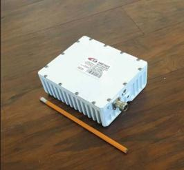
This smallest and lightest 15W L-To C-Band Block Up Converter is based on GaN technology. It is designed to be mounted on the feed horn. High power efficiency resulting in the low current (<1.5 amps @ 24VDC). The unit covers all three C-Band sub-bands: Standard (5.85-6.425 GHz), Palapa (6.365-6.725 GHz) and Insat (6.725-7.05 GHz).
