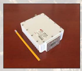
This smallest and lightest 15W L-To X-Band Block Up Converter is based on GaN technology. It is designed to be mounted on the feed horn. High power efficiency resulting in low current (<2A @ 24VDC).
