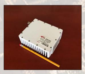
This smallest and lightest 15W(P1dB) L-T o C-Band Block Up Converter is based on GaN technology. It is designed to be mounted on the feed horn. High power efficiency resulting in low current (< 2.4 amps @ 24VDC). The unit covers C-Band sub-bands: Standard (5.85-6.425 GHz) and Palapa (6.365-6.725 GHz).
