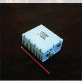
This smallest and lightest 12W L-To C-Band Block Up Converter is based on GaN technology. It is designed to be mounted on the feed horn. High power efficiency resulting in the low current (<=1.5 amps @ 24 VDC). The unit covers all three C-Band sub-bands: Standard (5.850-6.425 GHz), Palapa (6.365-6.725 GHz) and Insat (6.725-7.05 GHz).
