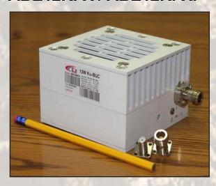
This smallest and lightest 12W L-To Ku-Band Block Up Converter is based on GaN technology. Incomparable low power consumption, double L.O., Field- Exchangeable connector and auto-ranging (24 or 48 VDC) powering features make unit universal for any Ku-Band application. M&C (FSK) capability enables troubleshooting, monitoring and controlling the BUC. User can choose internal 10MHz high stability reference if the corresponding modulator does not provide it.
