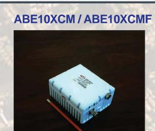
This smallest and lightest 10W L-To C-Band Block Up Converter is based on GaN technology. It is designed to be mounted on the feed horn. High power efficiency resulting in the low current (<=1.5 amps @ 24 VDC). The unit covers all three C-Band sub-bands: Standard (5.850-6.425 GHz), Palapa (6.365-6.725 GHz) and Insat (6.725-7.05 GHz).
