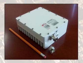
This smallest and lightest 10W L-To X-Band Block Up Converter is based on GaN technology. It is designed to be mounted on the feed horn. High power efficiency resulting in low current (<2A @ 24VDC).
