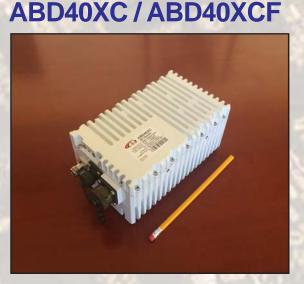
This smallest and lightest 40W(min) L-To C-Band Block Up Converter is based on GaN technology. It could be mounted directly on a feed horn. High power efficiency resulting in low current (<3 amps). The unit covers all three C-Band sub-bands: Standard (5.85-6.425 GHz), Palapa (6.365-6.725 GHz) and Insat (6.725-7.05 GHz).
