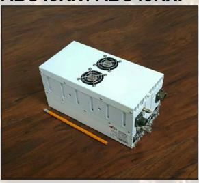
This smallest and lightest 40W L-To Ku-Band Block Up Converter is based on GaN technology. Incomparable low power consumption, double L.O., Field- Exchangeable connector and auto-ranging 36 - 58 VDC, or 80-240 VAC powering features make this unit universal for any Ku-Band application. M&C (FSK) capability enables troubleshooting, monitoring and controlling the BUC. User can choose internal 10MHz high stability reference if the corresponding modulator does not provide it.
