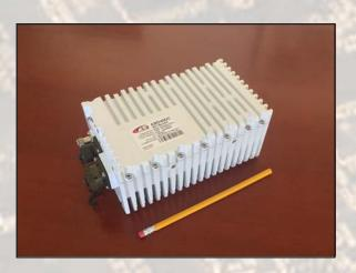
This smallest and lightest 40W(min) L-To C-Band Block Up Converter is based on GaN technology. It could be mounted directly on a feed horn. The unit covers Standard and Palapa C-Band frequencies: 5.85-6.725 GHz.
