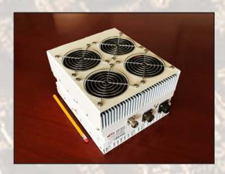
This smallest and lightest 150W L-T o Ku-Band Block Up Converter is based on GaN technology . Incomparable low power consumption, double L.O., Field- Exchangeable connector and auto-ranging 80-240 VAC powering features make this unit universal for any Ku-Band application. M&C (FSK) capability enables troubleshooting, monitoring and controlling the BUC. User can choose internal 10MHz high stability reference if the corresponding modulator does not provide it.
