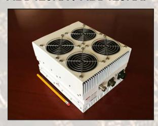
This smallest and lightest 125W L-T o Ku-Band Block Up Converter is based on GaN technology. Incomparable low power consumption, double L.O., Field- Exchangeable connector and auto-ranging 80-240 VAC powering features make this unit universal for any Ku-Band application. M&C (FSK) capability enables troubleshooting, monitoring and controlling the BUC. User can choose internal 10MHz high stability reference if the corresponding modulator does not provide it.
